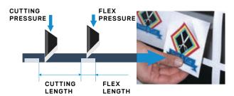
Alternately, one length is cut completely through the material, and one length is cut halfway through.
